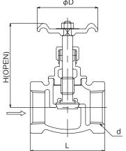
Wetted parts of GLV-16 are made of ductile cast iron. Widely applicable for steam, air, water or oil application.
