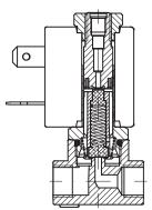
They can be **normally open (3/2 NA)** and in this case, at rest, the input orifice is open without electricity applied, the media reaches the intended use. Exhaust is closed.
