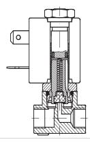
They can be **normally open (2/2 NA)**, in this case at rest the orifice remains open without electricity applied, the media reaches the intended use. When electricity is applied the input orifice closes
