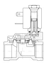
They can be **normally open (2/2 NA)**, and have an input and output connection machined into the valve body, and at rest the secondary plunger communicates with output, a minimum-pressure difference between the feed and the output causes the main shutter to rise, leading to it opening.
