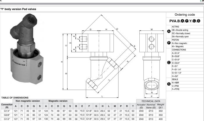
Pad valves, 2-ways, are a reliable and economic solution to control fluid. Pneumatically actuated by a compact double or single acting cylinder with 360° revolving connections. Standard seals in contact with fluid are made in NBR, FPM or PTFE. The barrel profile allows the use of Pneumax magnetic sensors series 1500 (see the Pneumax Genaral catalogue, chapter 4).
